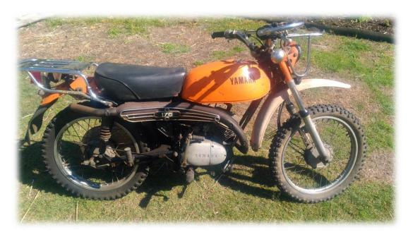
They were simple in design but developed after extensive testing. A basic single cylinder two stroke with auto lube (Yamaha's automatic oil in
